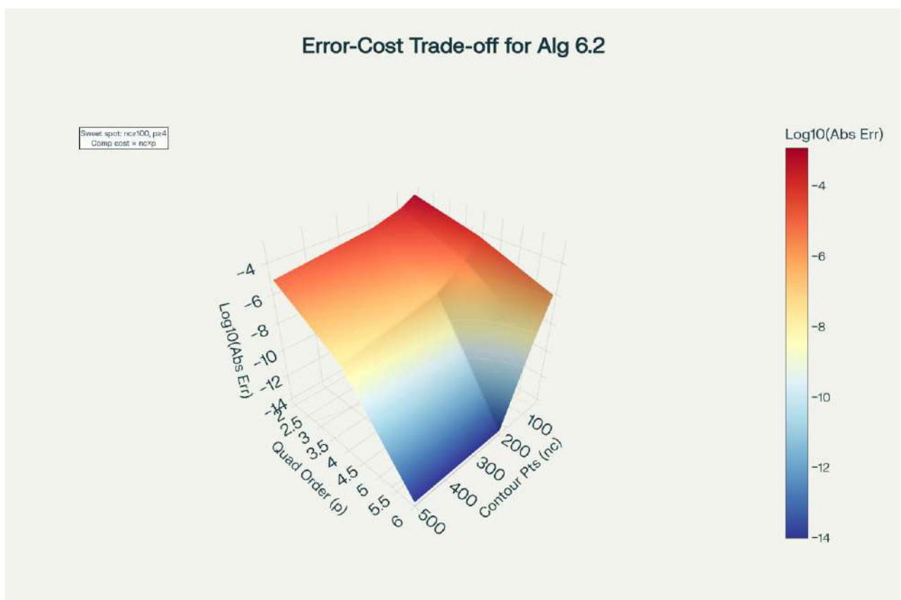
Figure 8: 3D surface (or 2D contour) of \log_{10} absolute error versus contour points and quadrature order for Algorithm 6.2, highlighting the sweet spot at higher p and moderate n_c
